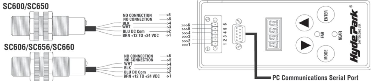
The SC660 has reversed outputs; a white-wire NPN and black-wire PNP output
